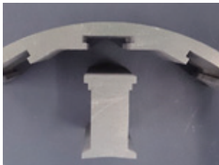
Fig. 4 Structure of Divided Core
