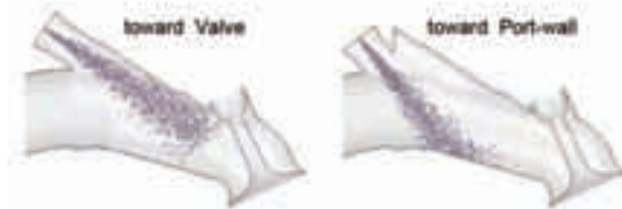
Figure 7: Configuration of injection
