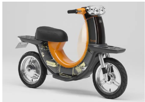
Fig. 6 Concept model "FC06" mounting a DMFC system
