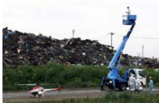
An operator controls the helicopter from a boom lift
