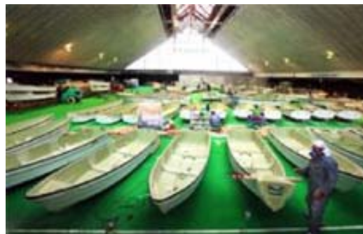
Boat hulls constructed by our group companies in Kumamoto, Hokkaido and Kagawa were sent to the "Sugo Outfitting Center" established on the tennis courts at Sportsland SUGO (facilities of a group company), where pre-delivery outfitting was carried out to suit the fishing methods of each region (Photo courtesy of The Yomiuri Shimbun)
